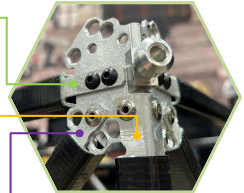
Partially riveted joint
