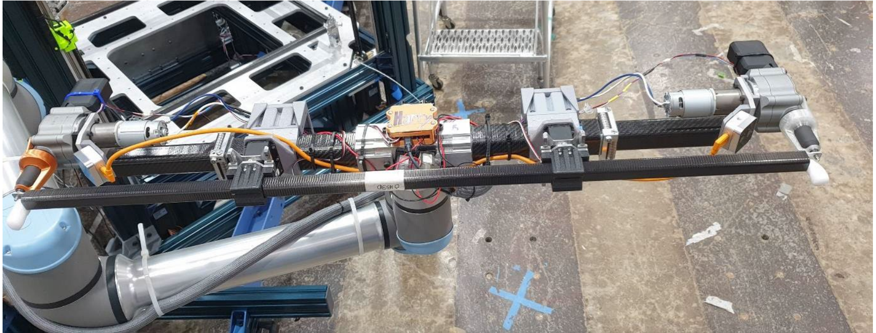
End effector mounted on UR10e
